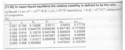
The relative volatility is a strong function of composition. It has a value of one for both components of a binary system at the azeotrope, and it is greater than one on one side and less than one on the other side.
